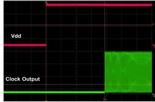
Figure 17. Startup Waveform vs. Vdd
